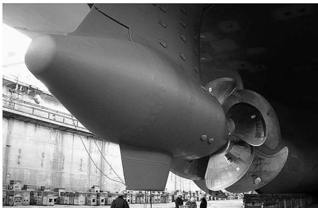
Fig. 1 CRP POD propulsion system
